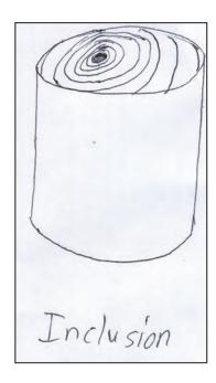
The other is inclusions inside metals. These failing points are caused by "junk" inside the metals causing a weakness internally. The "junk" could be oxides, molecules, or inter-metallic compounds.
