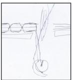
A presser foot is used to press down and slide the material along as the needle sews. After the two threads twist the needle rises and the material is moved which tightens the threads and sews the material together.
